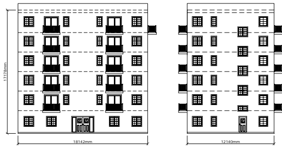
Figure 1: Elevation views of the six-storey test specimen
